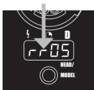
6. Select radio channel by turning the Energy Control D [13] until the desired channel is displayed in the Energy Display D [10]; for example channel 05 as in the figure above.
