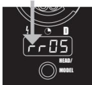
5. Set the generator to sync via radio by pressing the Head/Model Button D [12] until “r” is displayed in the second position in the Energy Display D [10]; see figure below. (If “-” is selected, sync via radio is not activated.)
